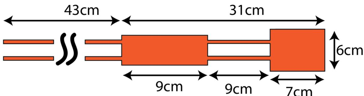
When selecting a Dewar to meet your needs, you must ensure that the mouth of the Dewar is wider than 6cm to allow the Cryostat to be lowered inside during its use. For the Dewar to be sealed with a Foam
