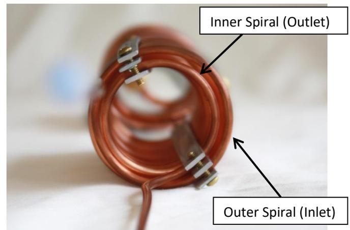
Prior to using the flow cryostat for the first time, it must first be purged with either Ultra High Purity Hydrogen or for 20 minutes to ensure that all moisture in the system has been removed. Moisture inside the cryostat will affect its performance. Purged gas should be vented to a fume hood for safety.
