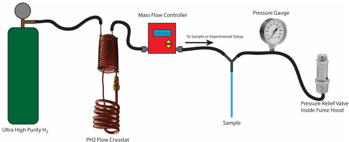
The figure above displays a typical experimental setup. For Initial Bench Top purging and testing, the sample is not required. Furthermore, for this bench top testing no cryogen is required.
